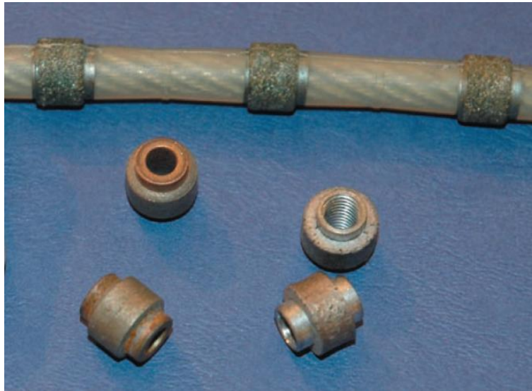
Fig. 9 Sintered beads and a wire saw used for sawing stone and concrete
