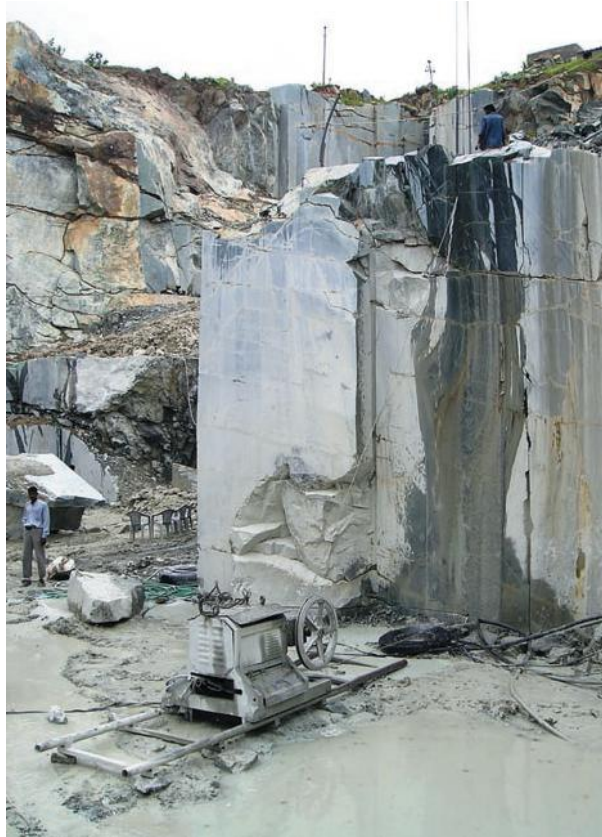
Fig. 15 Cutting a large block from the rock face (Courtesy of EHWA Diamond Ind. Co., Ltd.)
