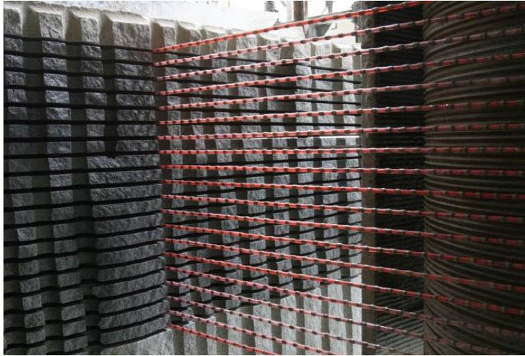
Fig. 17 Multi-wire machines are increasingly used for sawing thick sedimentary and metamorphic stone slabs, and as an alternative to the traditional steel shot gang saws used for granite block slabbing (Courtesy of Co.fi.plast. Srl).
