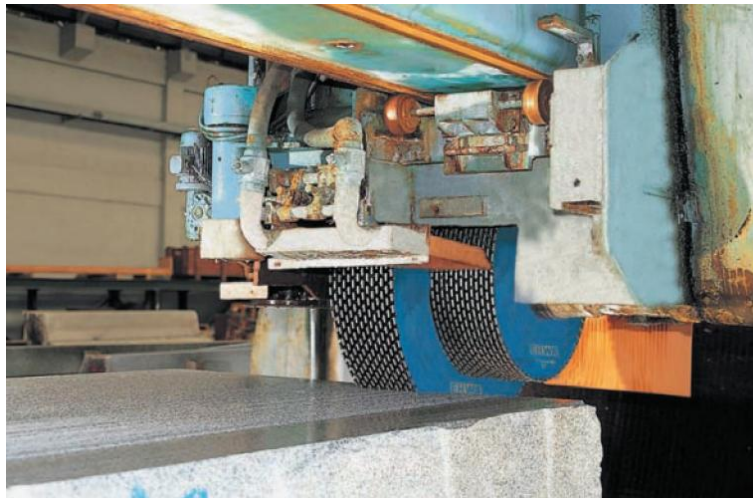
Fig. 13 Scaletta system multi-blade saw cutting a granite block (Courtesy of EHWA Diamond Ind. Co., Ltd.)
